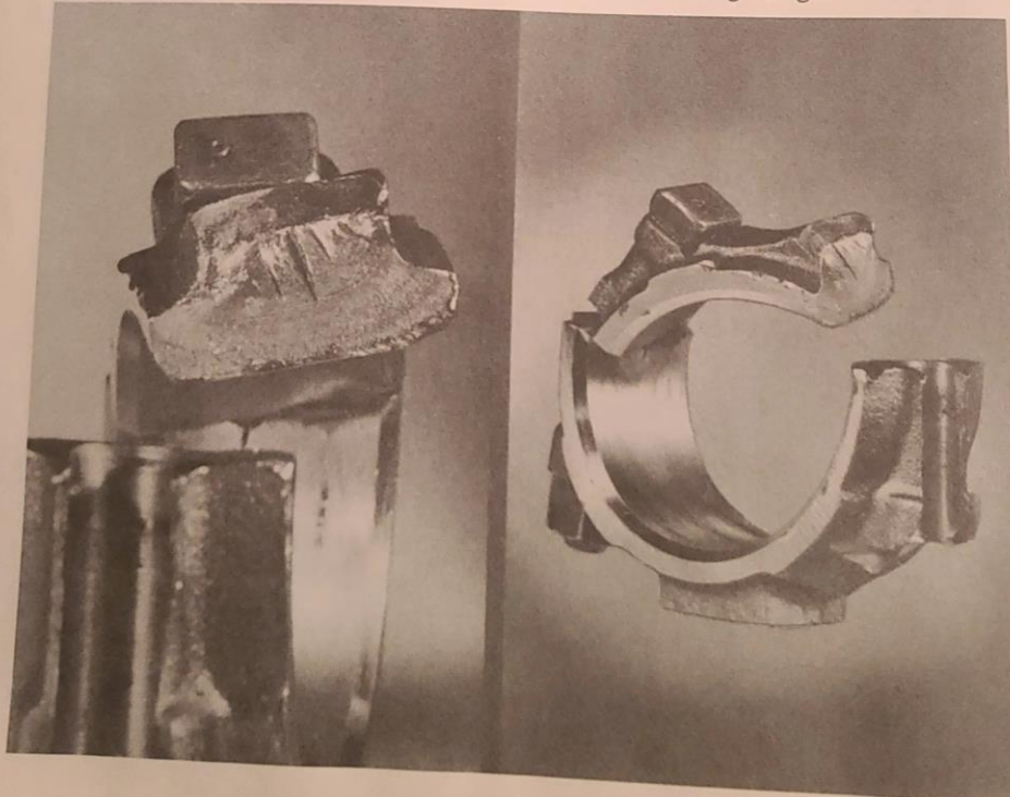
Component - connecting rod, Type Failure - bending fatigue
