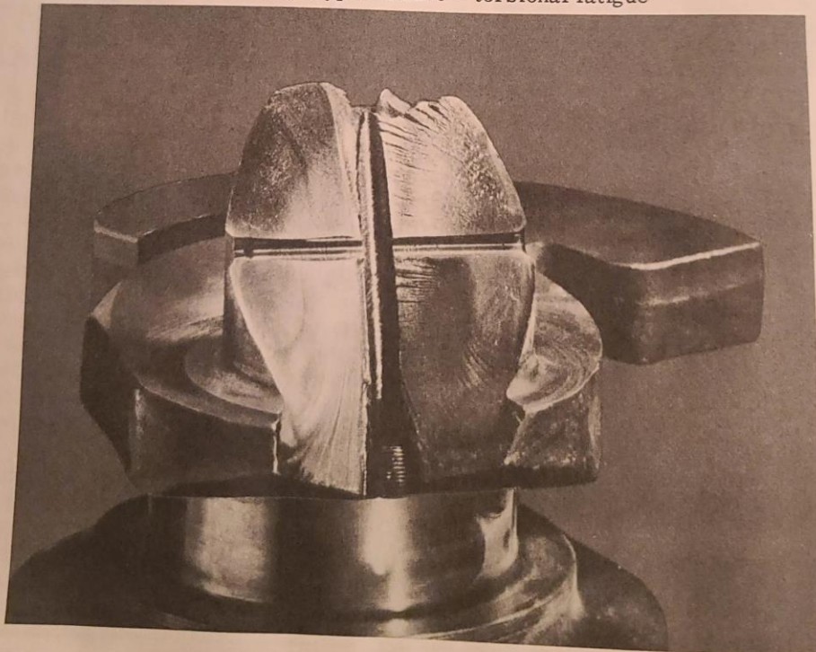
Component - crankshaft, Type Failure - torsional fatigue
