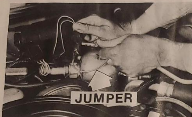
Fig. 31. Testing Park Switch
