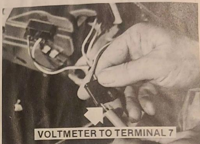
Fig. 55. Testing Variable Resistance for Voltage
