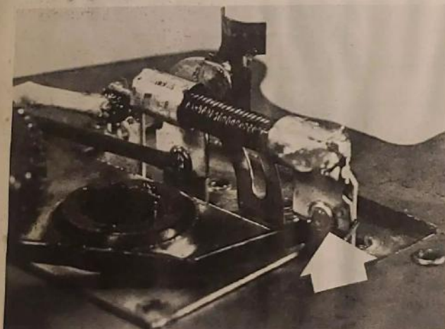
Fig. 14. Shunt Wire Connection
