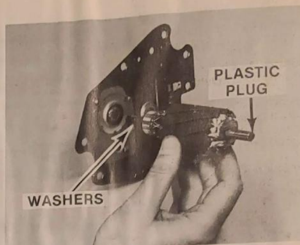
Fig. 12. Installing Armature
