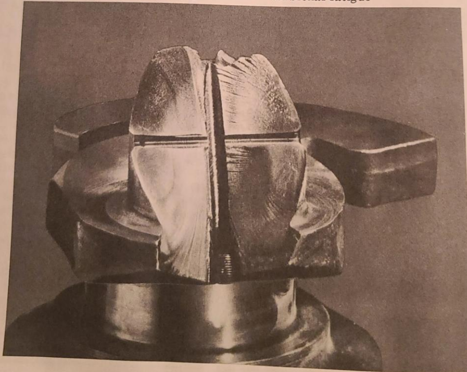
Component - crankshaft, Type Failure - torsional fatigue
