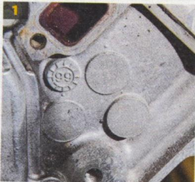
When trying to identify a block, one place to start is next to the water passages on the front. Many of the blocks like this LS1 have the year it was cast. Between the different LS1 castings, you typically want the later blocks because the machining improved over the years, not to mention the actual casting. The '99-and-later blocks featured added strength, thicker cylinder liners, and improved cam bearings, as well as better oiling.
