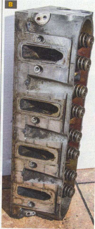
This is an original LS1 cylinder head—the cathedral port that started it all, carrying casting number 241. At 200 cc, the runner design is pretty high velocity yet still flowing 233 cfm at 0.600-inch. With porting, around 300 cfm can be achieved.
