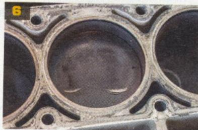
The 5.7L, by comparison, has greater support for each cylinder. However, for higher boost levels an iron block is still preferred.
