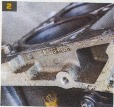
The oil passage is a dead giveaway, but if it is covered up—all early blocks carry casting number 12550592. This is an LS6 block, the most desirable 5.7L because it has improved crankcase breathing. It uses the same 319-T5 aluminum, centrifugally spun iron cylinder liners, powdered metal (steel) six-bolt main caps, and 3.89-inch bore. In case you are wondering, all OEM LS blocks have a 4.400-inch bore spacing and 9.240-inch deck height.
