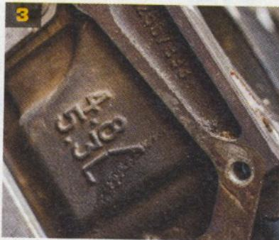
The engine size is also cast right into the front and rear of the block. From the factory, either the 4.8L or 5.3L would be circled with marker. Unfortunately over time it wears off and it is impossible to tell a 4.8L from a 5.3L from the exterior. The blocks are identical; it's just that the 4.8L has a shorter stroke crankshaft (3.267 vs. 3.620).
