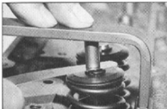
When performing a valve job on any Olds engine, a Mondello valve stem height gauge (#HG-455) is very important for correct rocker arm geometry and hydraulic lifter preload.
